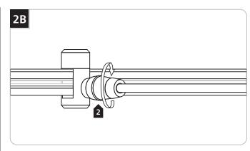
2 Tighten the FreeJack Fixture male connector.
