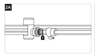
Push the FreeJack fixture male connector all the way into the Wall MonoRail fixture connector.
