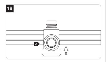
2 From bottom of the Monorail push the housing all the way onto the Monorail.
