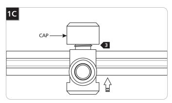
3 Replace and tighten the cap to the housing.
