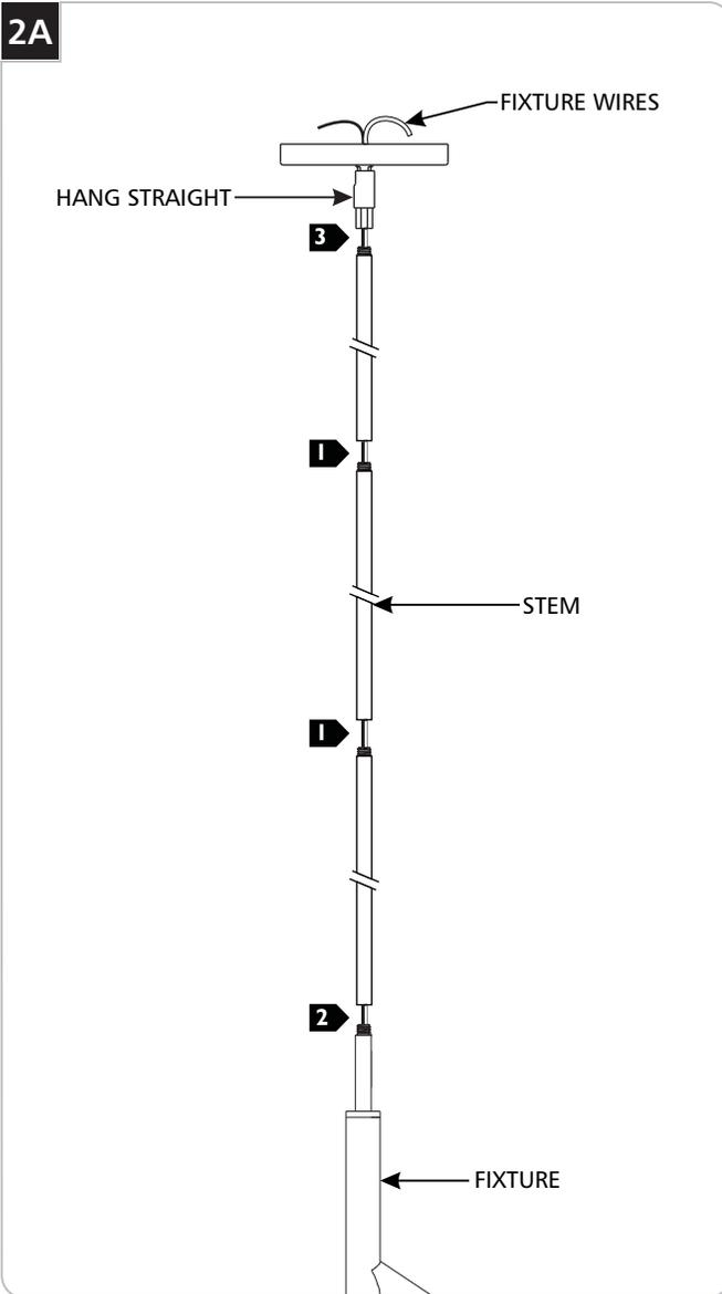
**NOTE:** This fixture can be mounted up to a 45° angle.
