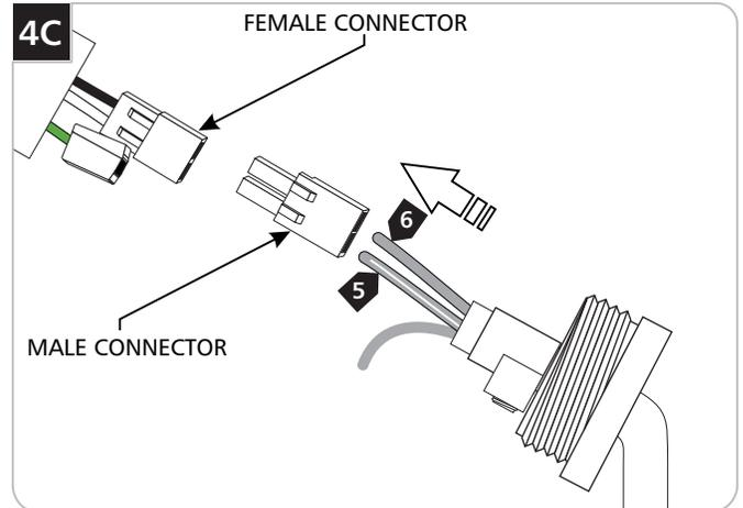
**CAUTION:** Exposed hot and neutral conductors may result in a short. Ensure no bare wire is exposed.
