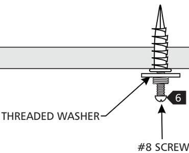
6 Screw the threaded washer onto the anchor with the long #8 screw.
