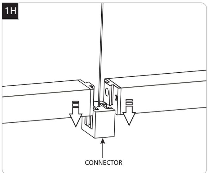
10 Slid one end of each fixture in to the keyed slot on the connector.
