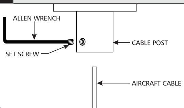
8 Determine the desired hanging height and cut aircraft cable to length.
