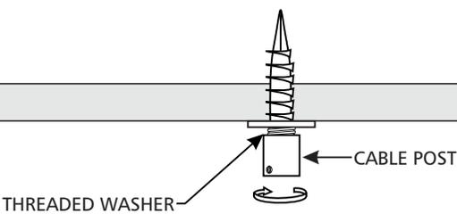
7 Tightly screw the cable post back onto the threaded washer.
