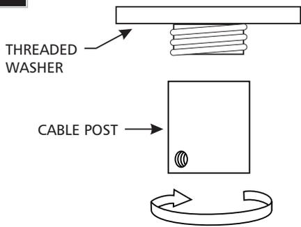
5 Unscrew the threaded washer to separate it from the cable post.
