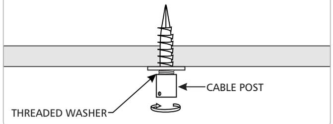
10 Tightly screw the cable post back onto the threaded washer.
