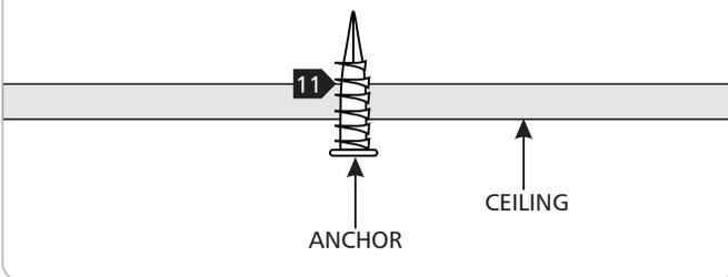
6 Tap the anchor at the marked point into the wall up to the threaded portion with a hammer.
