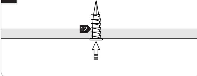
7 Screw the anchor in the rest of the way with a Phillips screwdriver.
