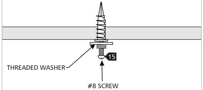
9 Screw the threaded washer onto the anchor with the long #8 screw.
