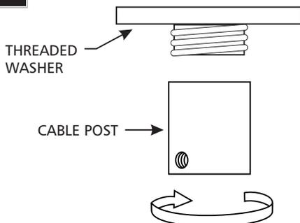
8 Unscrew the threaded washer to separate it from the cable post.
