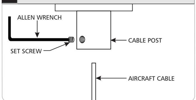
11 Determine the desired hanging height and cut aircraft cable to length.
