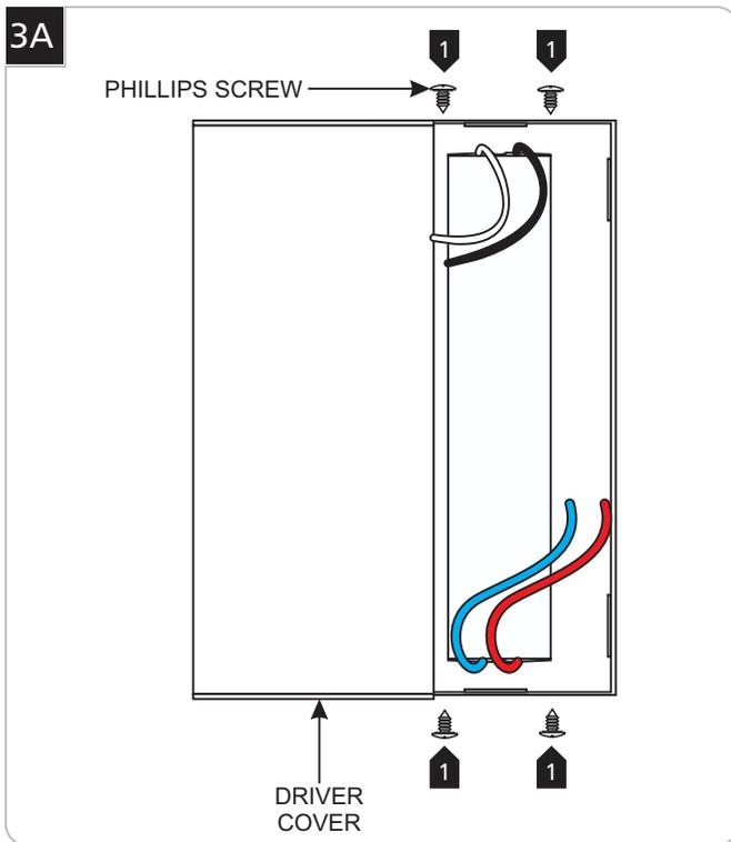
NOTE: For the 4' fixture the MAX wire length is 100ft from the driver to the junction box with 18AWG. for the 8' fixture the MAX wire length is 50ft from the driver to the junction box with 18AWG.
