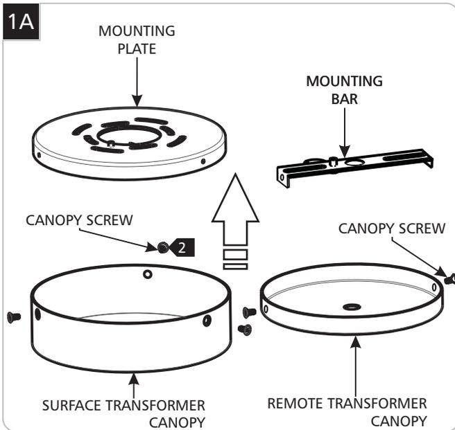
**1** Remove the screws from the canopy to remove the mounting plate/bar. (Three screws for the surface mount and two for the remote.)
