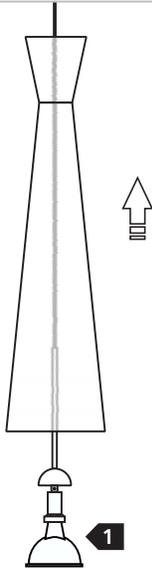
**1** Lift the shade up to expose the socket.
