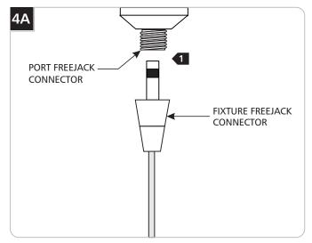
1 Tighten the fixture FreeJack connector completely into the port FreeJack connector.
