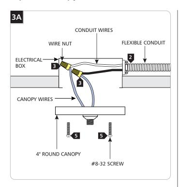
**NOTE:** Use the provided universal round crossbar when the canopy holes do not line up with the electrical box holes.
