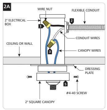
**NOTE:** The 2" electrical box must be installed prior to these steps. Refer to the instructions provided with the box.
