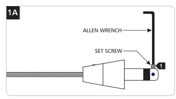
1 Back out (do not remove) the set screw on tip of the connector with the provided Allen wrench.
