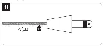
12 Pull the coaxial cable toward the fixture to smooth the wrinkles.
