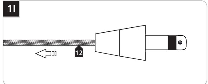
**12** Pull the coaxial cable toward the fixture to smooth the wrinkles.
