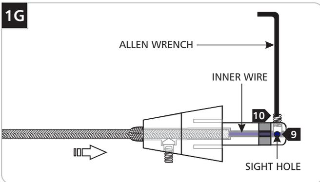
**9** Look into the sight hole on the top of the connector to make sure that the inner wire is contacting the end of the connector.
