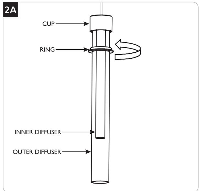
**1** Insert the inner diffuser into the cup followed by the outer diffuser, then slide the ring over the outer diffuser and screw it into the cup to secure in place.
