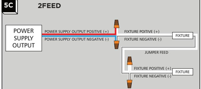
**NOTE: 2FEED fixtures are supplied with a jumper that can be used to power fixtures further down the run, that are separate from the initial run.**
