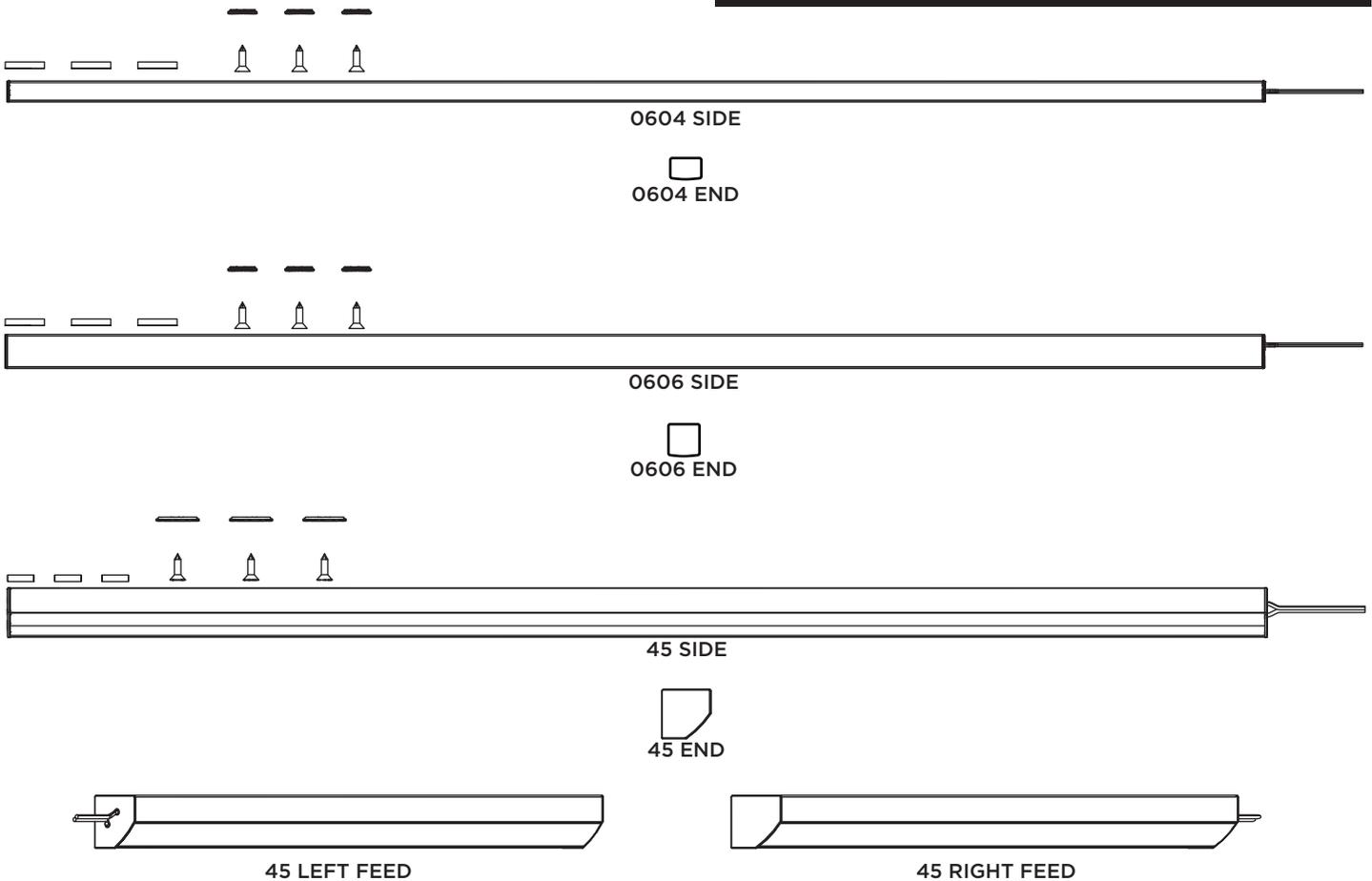
**NOTE: For the 45° fixture, the feed location is determined by viewing lens side of the fixture when installed.**
