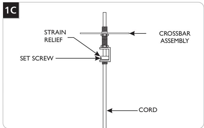
**4** Adjust the fixture height (from bottom of the fixture shade to top of the canopy) by moving the crossbar assembly up or down.
