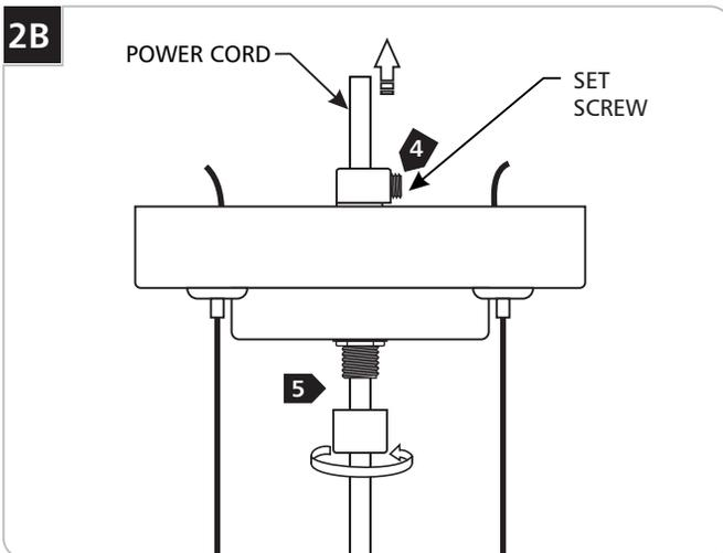
**Note:** Taping down the frayed end of the cloth cover may assist in feeding the power cord through the strain relief.
