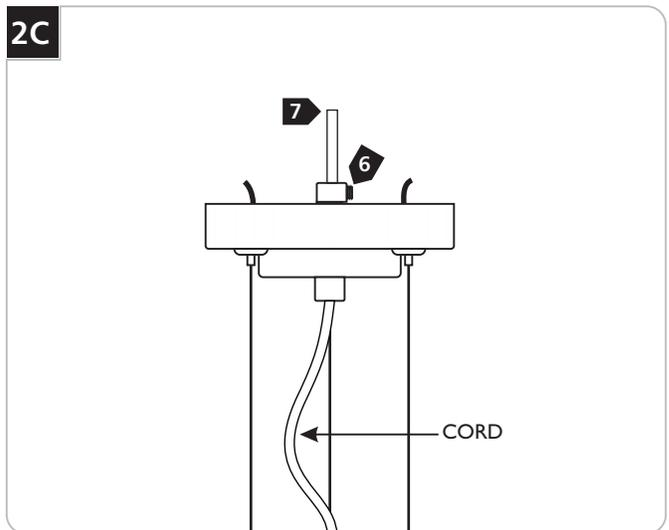
**NOTE:** The power cord does not support the fixture. For a casual "lazy cord" look, cut the power cord several inches longer than the drop height of the fixture.
