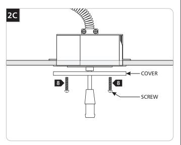
8 Mount the cover to the power feed port with the two #8-32 screws provided.
