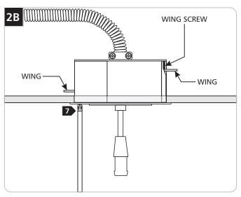
7 Tighten the two wing screws with a screwdriver until the wings secure the power feed port into the hole. An electric screwdriver will make this easier.
