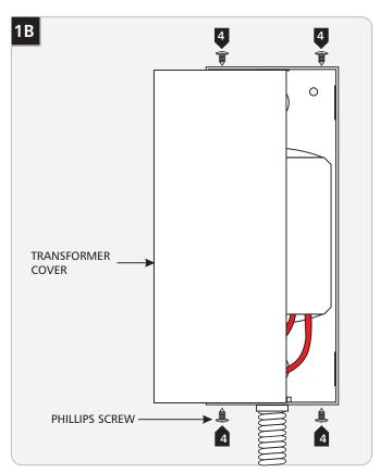
Remove the four Phillips screws to remove the transformer cover.
