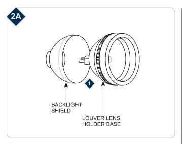
Push the backlight shield onto the louver lens holder base.
