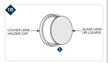
Place the louver or glass lens (optional-not included) into the louver lens holder cap.
