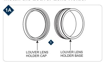
1 Unscrew the louver lens holder cap from the base.
