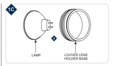
3 Place the lamp into the louver lens holder base.
