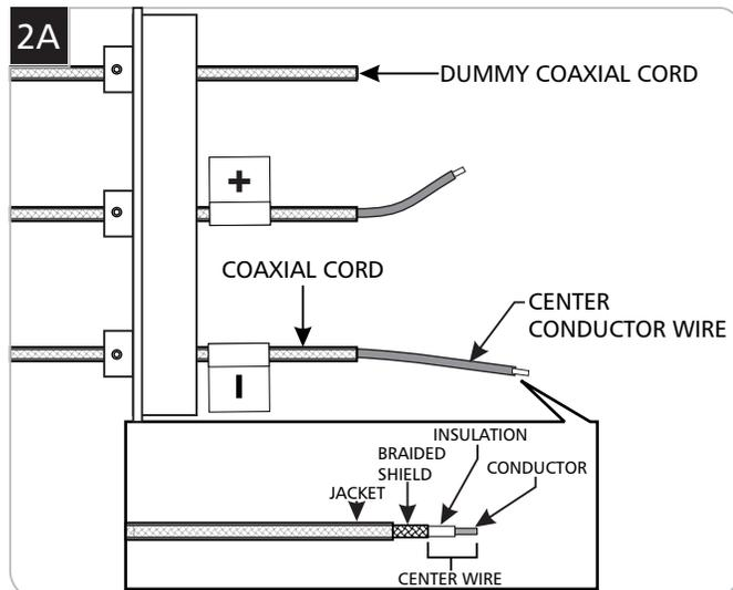
**NOTE:** If shortening is necessary, ensure that the cable identifiers are not removed during installation. If no shortening is necessary, skip to section 3A.
