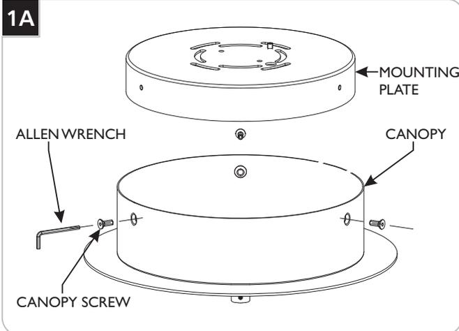
**1** Remove all the canopy screws from the canopy using the provided Allen Wrench and remove the mounting plate.
