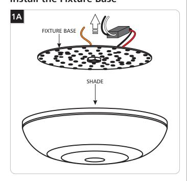
While supporting the shade, use a flathead screwdriver to separate the shade from the fixture base.
