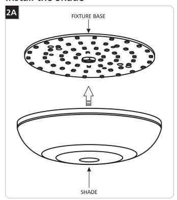
1 Install the shade by pushing it against the fixture base until it's secured with the magnets.
