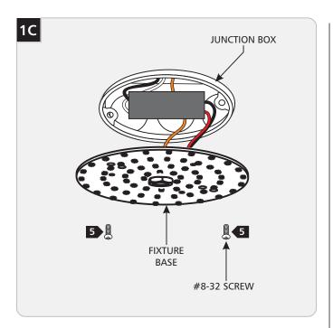
Properly place the driver, all wires, and wire nut connections into the junction box, secure the fixture base to the junction box with 2 #8-32 screws.
