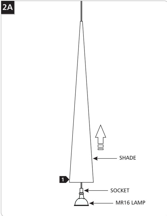
**1** Move the fixture shade up to expose the socket.
