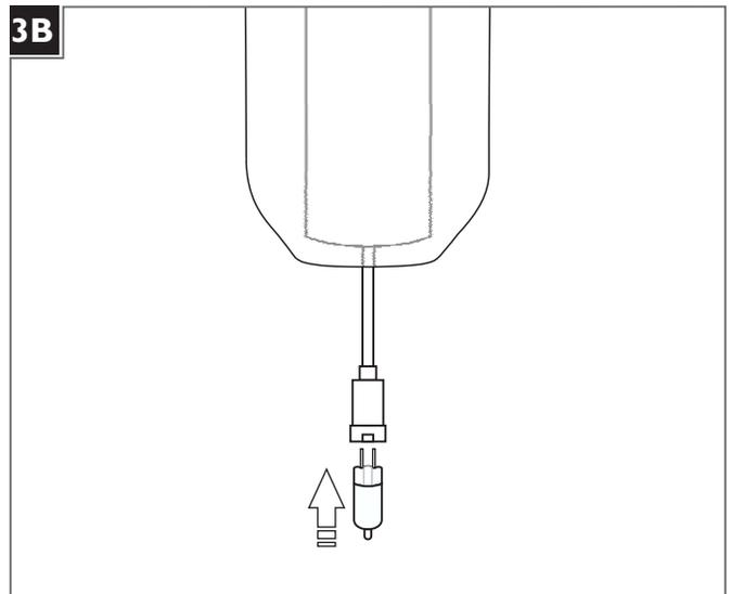
For incandescent versions, use **MAX 50 Watt** type frosted Xenon bi-pin lamp.
