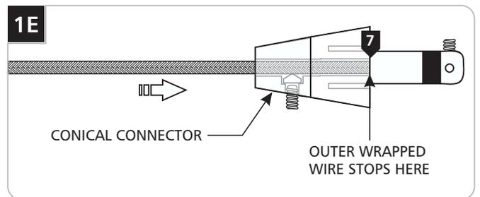
**7** Feed and push the coaxial cable into the conical connector. The coaxial cable will come to a stop point after being inserted 3/4" into the conical connector.
