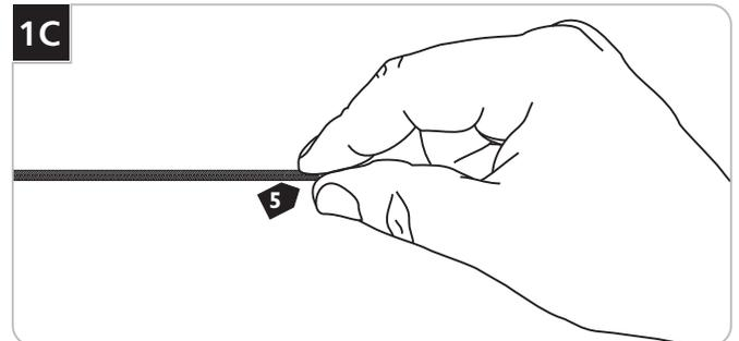
**4** Cut the coaxial cable to the desired length.
