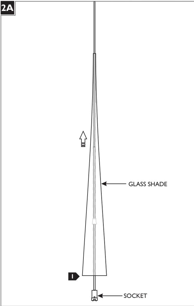
1 Lift the glass shade up to expose the socket.
