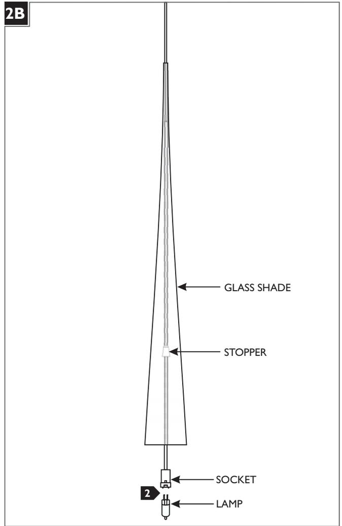
**NOTE:** To reduce the risk of a burn or electric shock during relamping, disconnect the power to the fixture.
