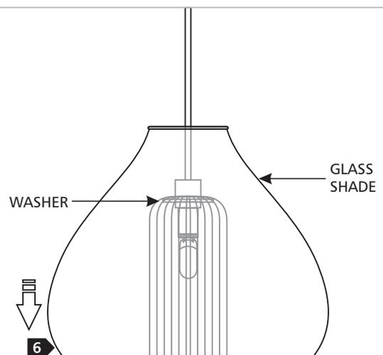
6 Carefully slide the glass shade down so that it rests on top of the washer.
